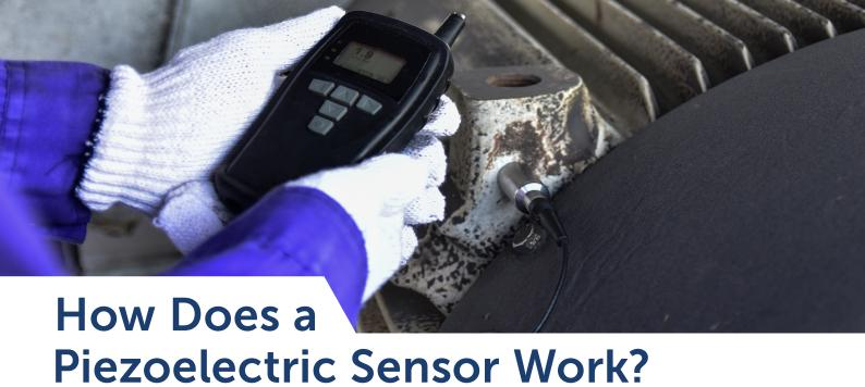
Piezoelectric sensors utilize the direct piezoelectric effect to convert a mechanical input into an electric signal. While the majority of piezoelectric sensors are based on the direct effect, some also exploit the converse effect as is the case with resonant piezoelectric sensors.
