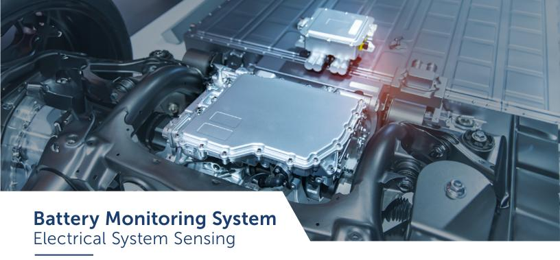
Battery Monitoring/Management Systems (BMS) are any electronic system that monitors the physical variables of a battery, such as current, voltage and temperature and prevents the battery from operating outside its safe operation parameters. Monitored variables are used to check the battery state, to calculate secondary data, report that data, control its environment, or for authentication
