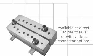
ESTIMATE Part Dimensions:  $64 \times 29 \times 16$  mm • <105 g (excl. connectors). Materials: Ag plated ceramic block with tin plated brass shield
