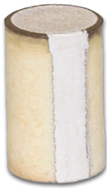
Transducer employing thick film applied on cylinder of porous ceramic
